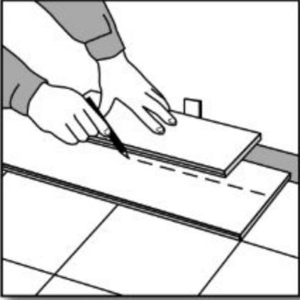
9) Use a full width scrap plank to mark your cutting line on the last row.
